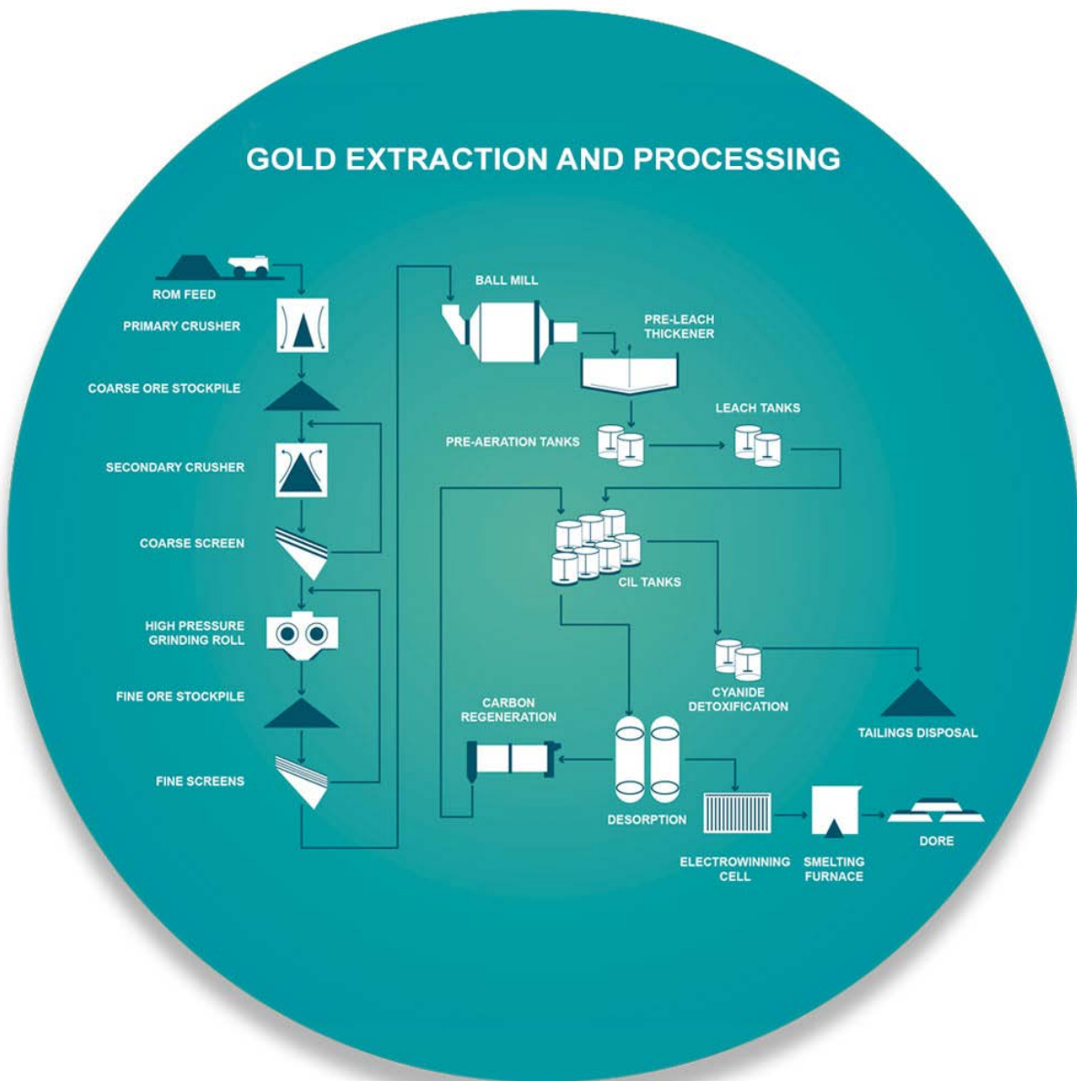
Figure 4 - Mining Production Process (Minerals Council of Australia, 2014)
